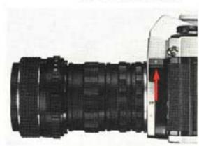
using any stop-down metering lenses. (Takumar lenses called just "Takumar", Auto-Takumar, Tele-Takumar and Super-Takumar are stop-down metering lenses.) When making a stop-down metering with your Spotmatic F, first focus the lens with the diaphragm fully open. Then, push up the stop-down lever and center the meter needle by turning the diaphragm ring or the shutter speed dial. You are ready to release the shutter.
