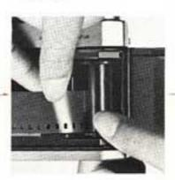
4. Cock the rapid wind lever, and confirm that the film rewind knob automatically turns counter-clockwise, indicating that the film is properly loaded and is moving from cassette to take-up spool, Trip the shutter.
