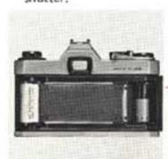
5. The first portions of the film cannot be used for picture taking as they have already been exposed to light, Generally, two or three blank exposures should be made before taking your first picture. Therefore, advance the film until the exposure counter turns to "1", indicating that the first picture is ready to be taken.
