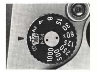
The ASA film speed rating of all 35mm films is given in the data sheet packed with each roll of film. The higher the ASA number, the more sensitive the film. Lift the outer ring of the shutter speed dial and rotate it until the ASA number of your film is opposite the orange dot alongside the figure 1.
